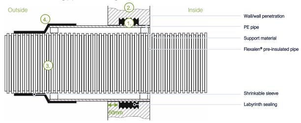
Clean the PE pipe and slide the labyrinth seal over the clean pipe. Slide it through the wall penetration and position it centrally with a horizontal distance of the wall seal from the outside wall of approx. 60 mm.
