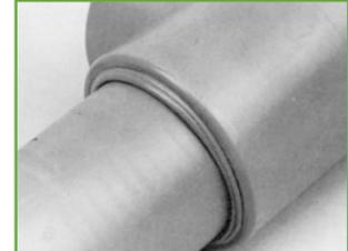
**12.** Visible check: Two beads (of pipe and fitting) are visible. Correct alignment of pipe and fitting. Marked insertion depth is visible.
