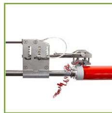
b) Remove the oxygen barrier with our Flexalen PB EVOH Scraper up to the marked insertion depth (should remain visible).
