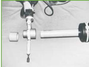
**09.** Bring the welding device, pipe and fitting into position.
