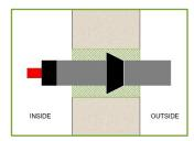
To seal the wall penetration, backfill the carrier pipe and labyrinth seal centrally positioned with commercially available swelling mortar (concrete).
