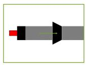
Clean the casing of the pre-insulated pipe and slide the labyrinth seal over the clean pipe.
