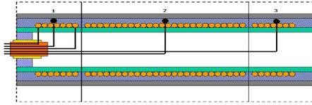
Figure 1, Longitudinal section guarded end heating probe
