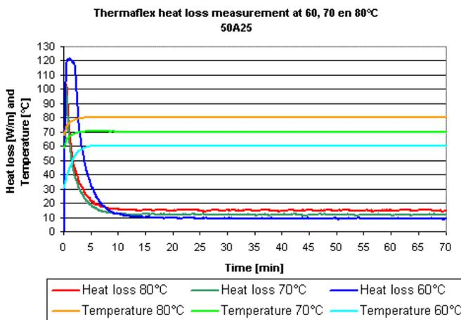
Graph 2, Power and temperature of the heating probe
